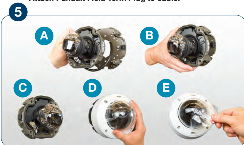
Route cable to avoid bends, mount camera and apply cover.
